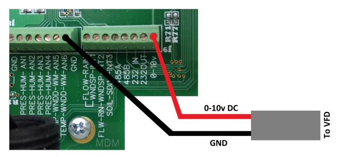
0-10v DC Terminal of the Crop Link unit as shown goes to the VFD 0-10v DC input
