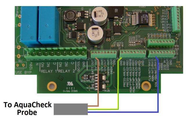
Wiring the AquaCheck probe: Only 1 probe can be connected to this unit at a time.
