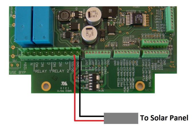
Wiring the solar panel: Find the last two terminals on the large terminal strip labeled DC/SOL and GND
