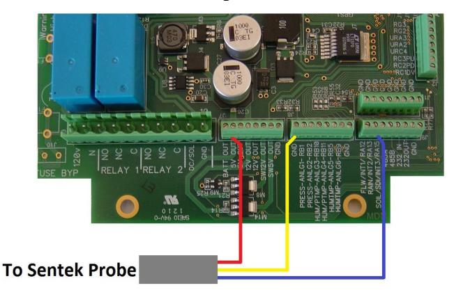
Wiring the Sentek probe: Only 1 probe can be connected to this unit at a time.
