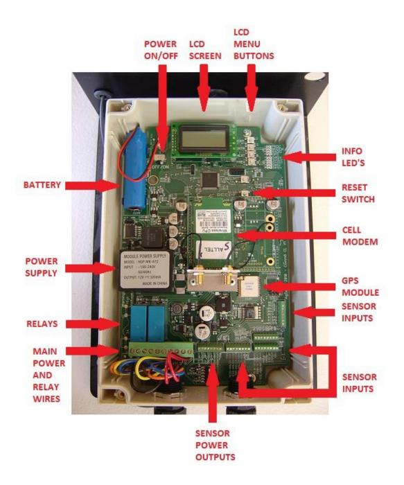
Note: Once all sensors are connected and unit is ready to run, contact your AgSense Dealer to finish setup, and configure this unit to read the sensors that you have installed.
