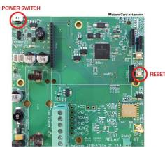
5. Hold in the RESET button while turning on the Power Switch. (see red circled areas)
