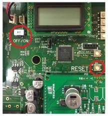
Hold in the RESET button while turning on the Power Switch. (see red circled areas)
