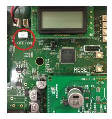
2. Turn the Power Switch to the 'Off' Position.
