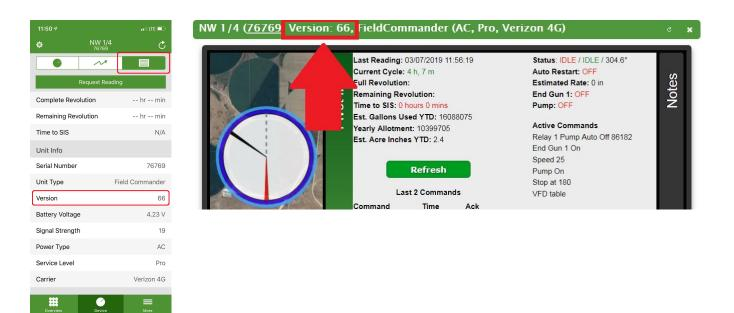
1. AgSense devices require a minimum firmware version of 66 for the new Telit 4G modem/d-card to be compatible. If the firmware is less than 66, an update is required before continuing to the next step. Please call AgSense at 605-352-8350 with the device serial number. The device must have power and be communicating for the update to download. The firmware is visible on the AgSense App in the 'Pivot Info Tab' and on the web on the 'Pivot Info' Screen.
