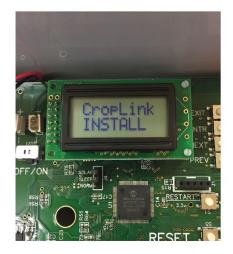
Wait for the unit to do its self-checks, and finally say CropLink (or appropriate device) INSTALL.
