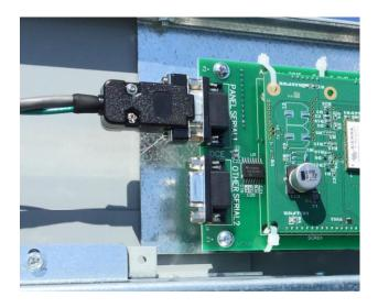
Connect the opposite end of the Serial Cable to the Valley panel 9 pin Serial Port on the panel door as shown in the photo below.
