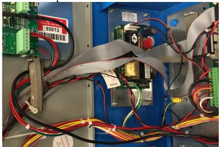
4. Then screw the antenna cable end onto the cell modem card as shown in the photo below (gold screw connection)
