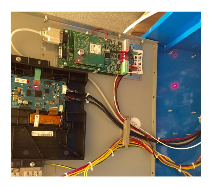
Connect the opposite end of the Serial Cable to the Valley panel 9 pin Serial Port (J12) on the SRB Relay board in the panel as shown in the photo below.
