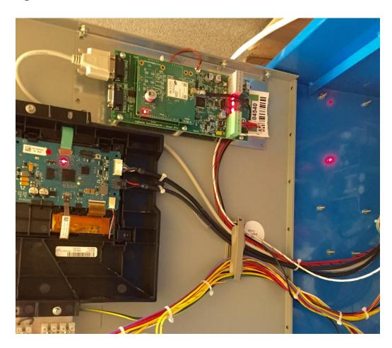
3. Then screw the antenna cable end onto the cell modem card as shown in the photo below (gold screw connection)
